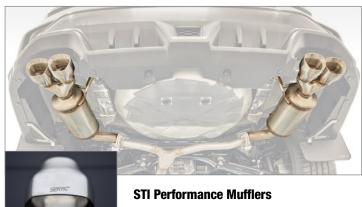
Manufactured from 304-stainless steel and debossed with the STI logo, the STI Performance Mufflers feature double-walled, hexagonal guad tips to create a sleek appearance and aggressive growl. They are lighter weight for easy direct bolt-on installation and have less back pressure than the stock mufflers.
