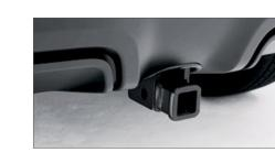
Accessory Activity Mount. With its durable steel construction, the Accessory Activity Mount allows you to carry up to 100 lbs. of additional gear. It's also designed and tested to be an integral safety component as it replaces the vehicle's rear bumper beam.
